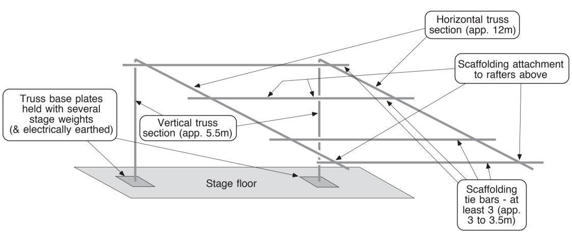
All trussing is LITEBEAM 'SLICK' TRUSSING as supplied by Northern Light, and has a safe working load of 320kg (evenly distributed) for a 7m span without supports (the longest span in this case) incorporating a 3:1 safety factor.
